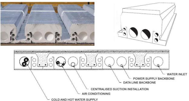
Floors and roofs in ICF - Insulated Concrete Form system
