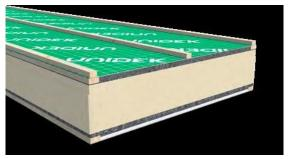
Aero Comfort is an insulating sandwich element with a core of EPS Platinum, fire retardant modified, equipped with 4 integrated stiffeners of 19 mm high and 45 mm wide. The outside is provided with a 3 mm chipboard with green foil and diamond pattern and 3 battens of 20 mm high and 30 mm wide. The inside is provided of a 12 mm plasterboard, which is between two stiffeners applied, finished with a 3 mm chipboard provided of a white visible side.
