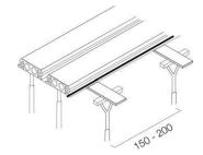
One of the most important and unique product properties is the continuous insulation, which is ensured partly by the connection with male / female profiles. The thickness of the floor slab can be kept to an absolute minimum and the U values can easily drop to 0.17 W/m<sup>2</sup> K.
