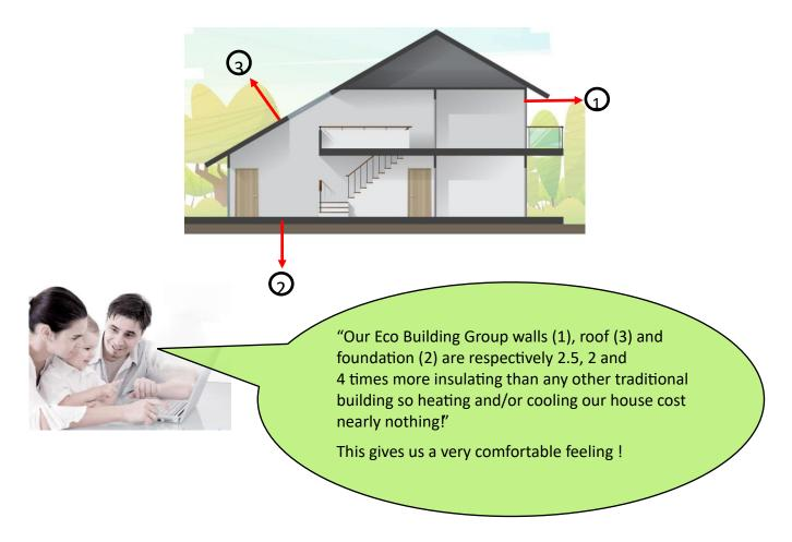
The Eco Building Group construction method can be compared to a lost formwork, however limited to the creation of a construction in reinforced concrete. The formwork, made of hard insulation material, serves as an insulation of the new erected concrete wall, and this on the internal and external side. We supply a full range various coordinated elements, in different thickness for both the insulation layer as the concrete core.
